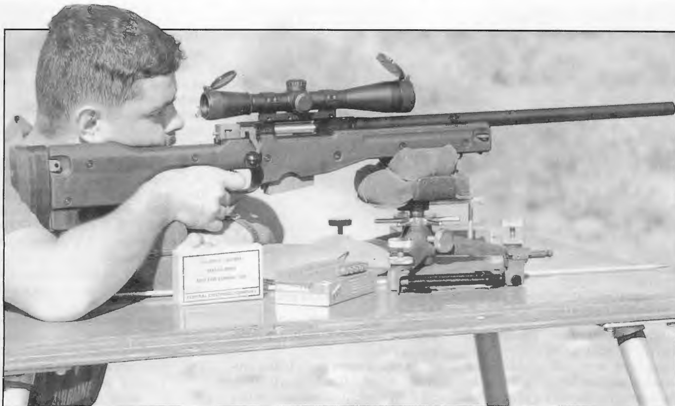
AWP rifle with its heavy match barrel, Leupold Mark 4 M3-10X scope and Federal 308M ammunition will consistently shoot sub-1/2 MOA groups.
